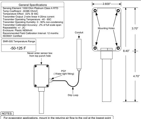
For evaporator applications, mount in the returing air flow to the coil at the lowest point possible.
