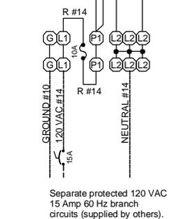
Separate protected 120 VAC 15 Amp 60 Hz branch circuits (supplied by others).
